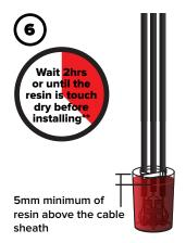
As soon as the resin begins to mix within the nozzle the user must start to fill the containers, the user will have **2** minutes\*\* to extrude the mixture. Pot a minimum of 5mm above the end of the cable sheath to ensure IP68 rating.
